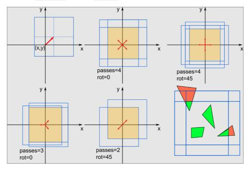
Note: Beamfox Proximity will display the effective write field instead of all the individual multi-pass write fields. This results in a virtual write field that is smaller than the specified size.
